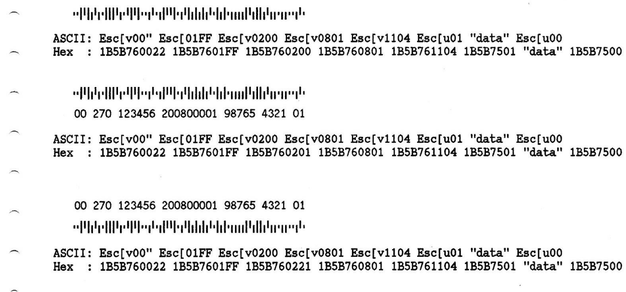
Figure 72. Intelligent Mail Bar Code in Epson/IBM Commands Example (Bar Code Mode Alt. 1)
